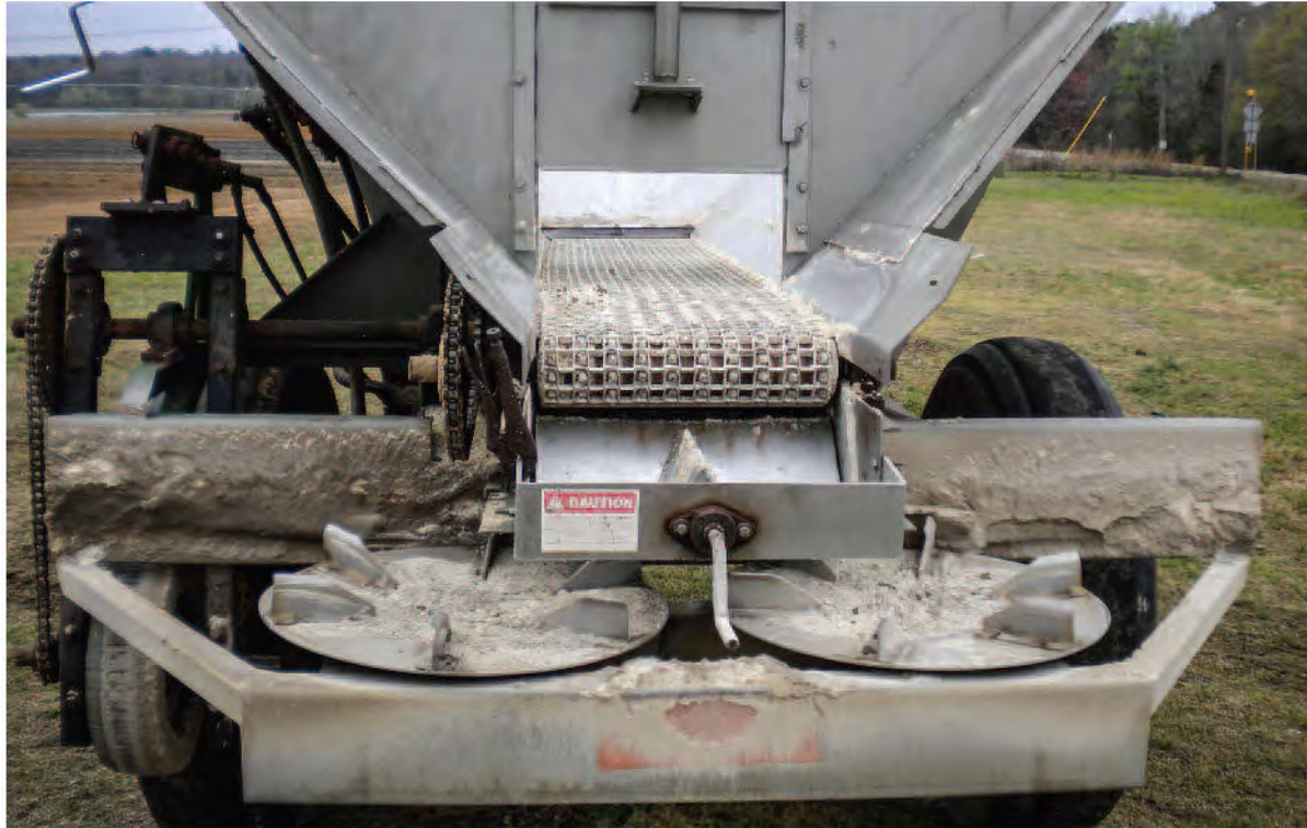
This is the distribution mechanism of a lime spreader. Notice the conveyor chain that moves dolomitic limestone out of the hopper. The dolomitic limestone falls onto a pair of circular, rotating distributors that spread the material in a wide swath. The hydraulic system of the tractor powers this spreader.
