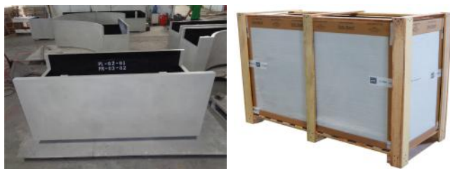
One of the GRC elements during the manufacturing stage and after packing
