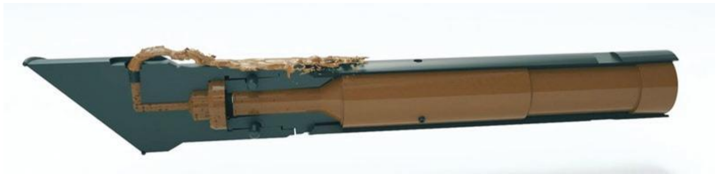
Bentonite lubrication moves through the outer ring of the dual-wall pilot tube to the steering head port to reduce jacking forces as the steering head displaces the ground.
