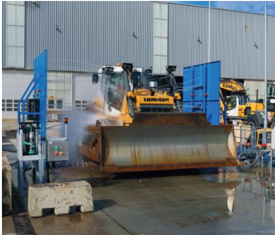
The MobyDick demucking system from Frutiger
