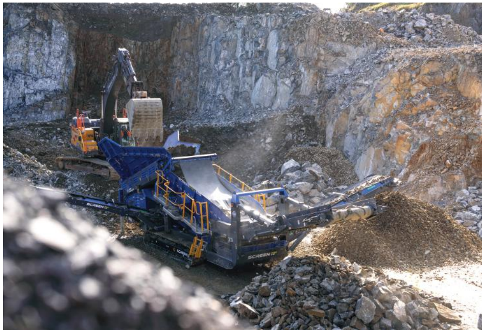
The EDGE Screenpro S18 heavy-duty, tracked scalping screen
