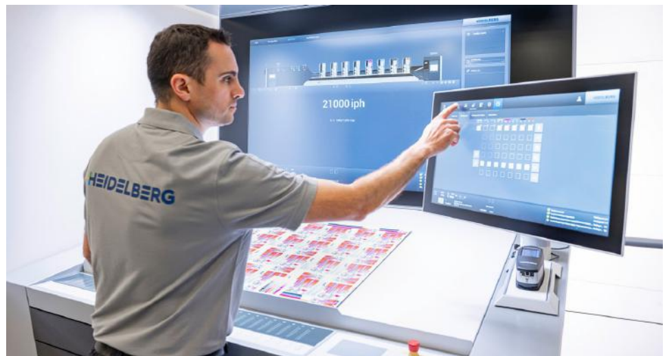
The highly automated Peak Performance Speedmaster XL 106 with up to 21,000 sheets per hour on show at drupa 2024 enables autonomous print production.
