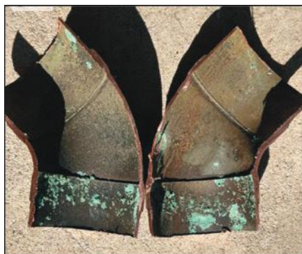
Figure 6 The distinctive appearance and location of these marks suggest they result from cavitation events rather than typical erosion-corrosion (photo courtesy of Phil Woolhouse)
