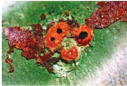
Figure 1 Typical soft water pit from Evans Head, NSW, showing coarse cuprous oxide (photo courtesy of Dr David M. Nicholas)
