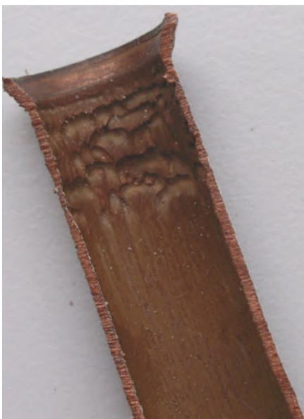
Figure 4 Deeply 'scalloped' pipe surface, typically near pipe joint. (photo courtesy of Dr David M. Nicholas)
