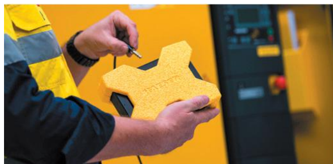
Image 2; The air demand can be precisely calculated and evaluated using modern measuring devices such as the ADA data loggers from KAESER (for analysing compressed air duty cycles).
