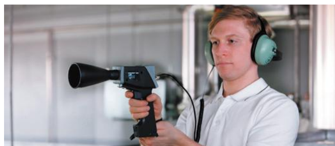
Image 5; Leaks should be measured regularly. Pictured above an Ultra Sonic Leak Detector (USLD).
