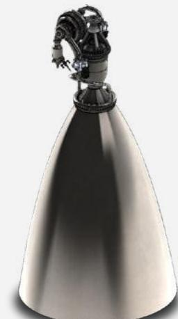
The RS-2 is a bipropellant liquid rocket engine with a single regenerative cooled thrust chamber, fed in pressurized form. It was used as a test platform for swirl injectors, ignition characterization, and evaluation of thermal loads on cooled thrust chambers. The thrust chamber was manufactured using a combination of additive technology and electroforming.
