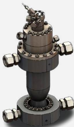
The RS-2 is a bipropellant liquid rocket engine with a single regenerative cooled thrust chamber, fed in pressurized form. It was used as a test platform for swirl injectors, ignition characterization, and evaluation of thermal loads in cooled thrust chambers. The thrust chamber was manufactured using a combination of additive technology and electroforming.
