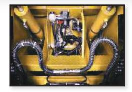
**ELECTRICAL PANEL:** Electrical, steering, and brake maintenance is facilitated through a hinged compartment located at the front of the unit.
