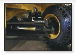
**STEERING CONTROL:** Designed for durability and performance with an oversized axle featuring high steer angle and heavy duty spindles.
