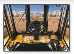
**CLOSED CAB:** The all-weather closed cab option is equipped with sound insulation, defroster fan, heavy duty heater, window wipers, removable 2-piece split doors with sliding windows, and 360 degree visibility for safe, efficient, and comfortable operation.
