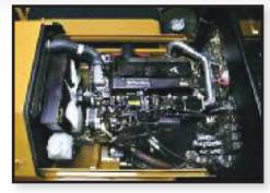
**ENGINE:** The unique sliding hood provides unobstructed engine access for quick maintenance checks. A Perkins Tier 4 Turbo Diesel is standard.
