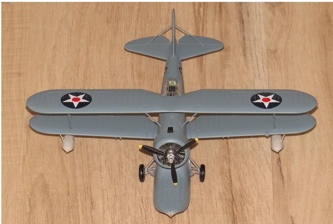
This angle of the Easy Model 1/48 scale Grumman J2F-5 Duck highlights some of the unique design features of the aircraft, including the stabilizing floats mounted on the lower wings, the externally braced tailplane, and the landing gear that retracted into the central float. Easy Model did an excellent job replicating these features on their J2F-5 Duck.
