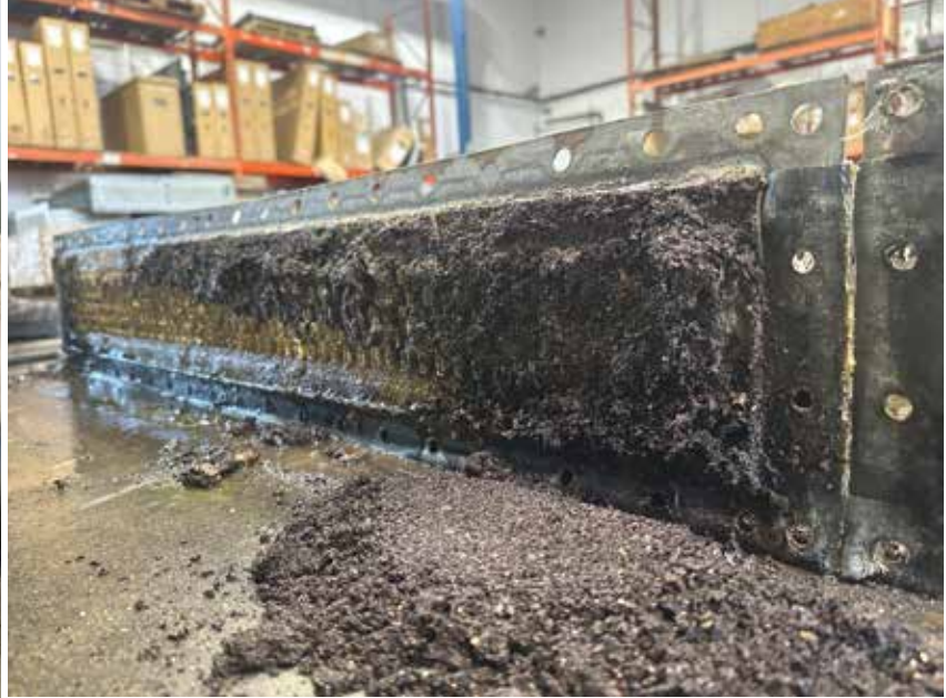
A clogged and corroded back-up generator heat exchanger – the kind of issue West End Rad's custom-manufactured aluminum coolant reservoirs are designed to prevent.
