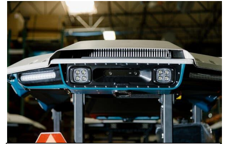
Figure 20: Cameras and sensors in the roof help gather data.
