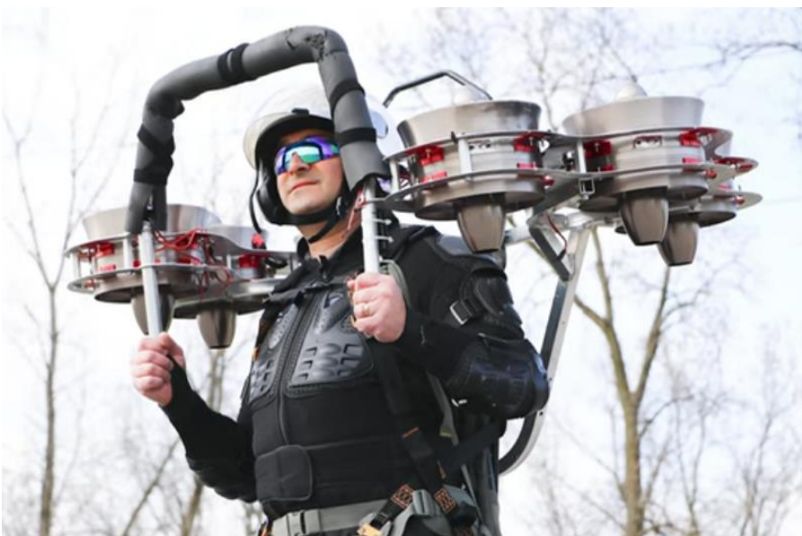
Figure 15: Electric Jet Aircraft's EJ-1H Jetpack uses six battery powered ducted fans to provide more than 320 lbs of thrust to carry a 200 pound pilot. The EJ-1 has gone through several variations and proof-of-concepts since 2019. Electric Jet Aircraft hopes their jetpack will be used for anything from air shows and personal use to first responders. 60
