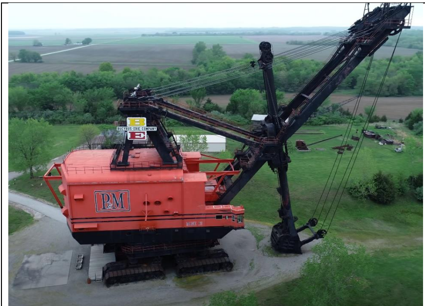
Figure 19: Bucyrus-Erie model 1850-B, AKA “Big Brutus”, the largest existing electric shovel in the world.
