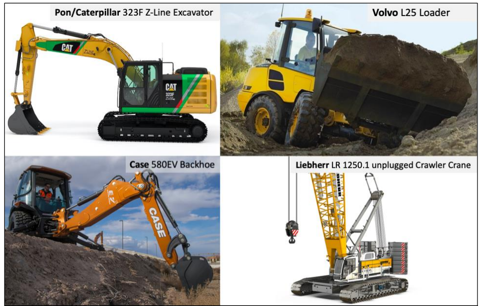
Figure 8: Electric options for heavy equipment are becoming more available.
