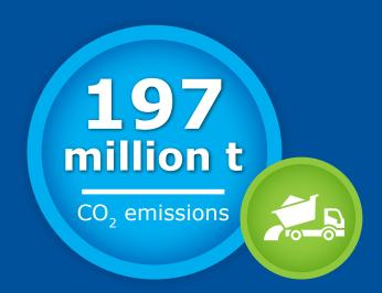
Through the use of granulated slag in place of Portland cement clinker in cement, the emission of 197 million tonnes of CO<sub>2</sub> could have been avoided since 1949.
