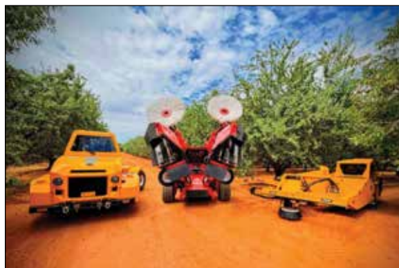
Bonsai Robotics retrofits orchard machinery (like nut tree shakers and sweepers) with advanced vision and control systems, turning them into self-driving machines.
