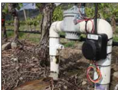
Verdì combines easy-to-install hardware (wireless valve controllers and sensors) with a farmer-friendly software app to automate irrigation at scale. Photo courtesy of Verdì
