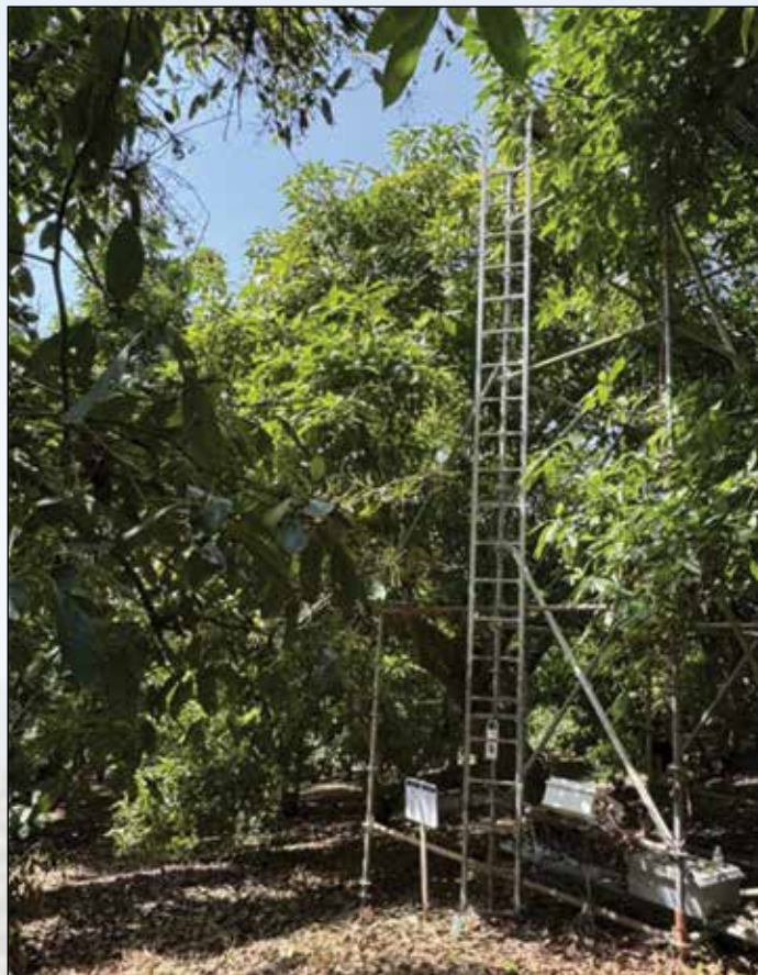
Sensors mounted on towers high above the avocado orchard canopy were crucial in collecting real-world data for more precise crop coefficients.
