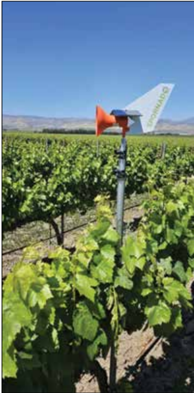
The Spornado sampler is a passive spore trap that detects crop disease pathogens in the air long before symptoms appear on plants.
