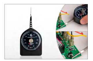
**Small Force Gauges** (Flat Tip, Dial Diameter 1 1/2")
