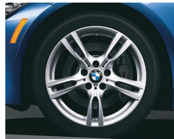
Star Spoke light alloy wheels (Style 400M) 18 x 8.0 front, 18 x 8.5 rear; and 225/45 front, 255/40 rear run-flat 1 performance tires 2,3 18 x 8.0; and 225/45 non-run-flat 1 all-season tires 2
